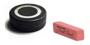
Elastomers have an inherent hardness because of their chemical structure. This hardness can be modified, and the processed hardness then measured in terms of durometer (duro) on a Shore scale.
